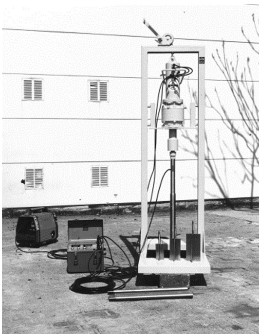
Fig. 10 Vane blades and driving frame for testing in boreholes [83]
